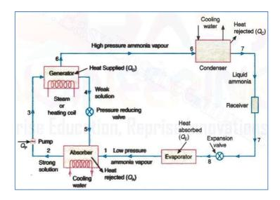
Fig.1 Schematic Diagram of Vapour Absorption Refrigeration System [10]
