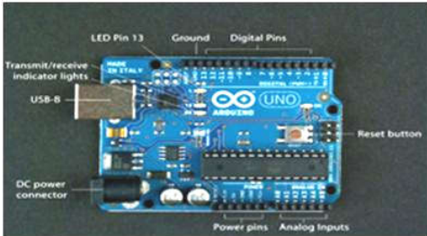
Figure 1: Arduino Uno R3 board ATmega328P
