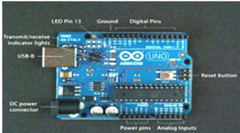
Figure 1: Arduino Uno R3 board ATmega328P
