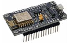
Figure 2: ESP8266 Node MCU
